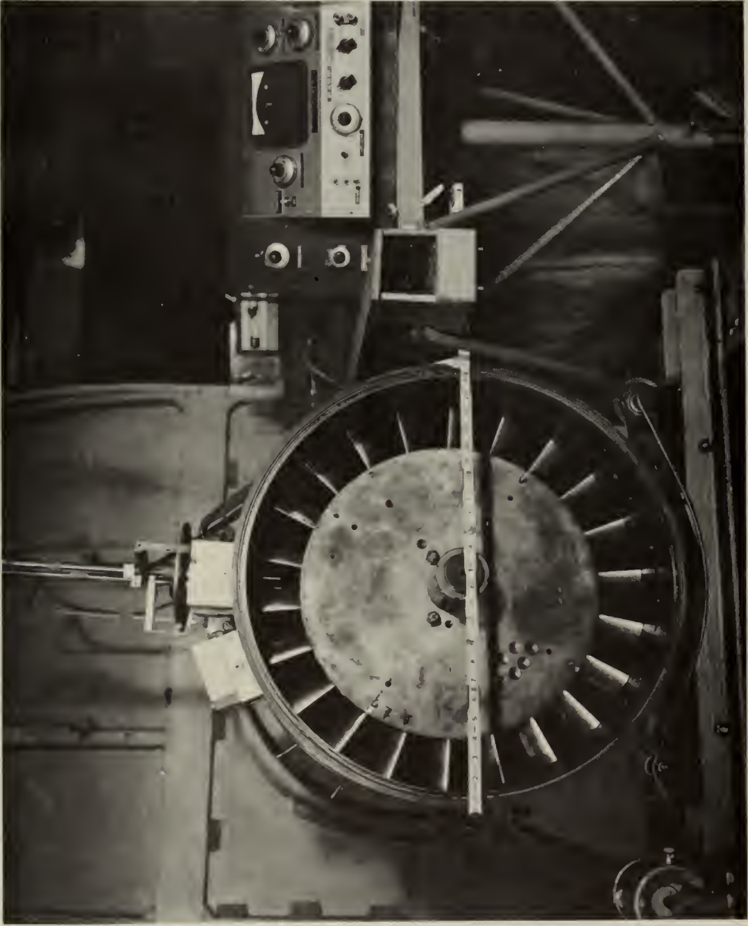
FIG. 2 VIEW OF ROTOR (2b/S=0.525) WITH CASING REMOVED
