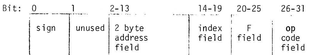
One alternate technique considered was to store each MIX word in a 6 byte 360 packed format. This would have required an additional 8000 bytes of 360 core to simulate a 4000 word MIX computer. The 32 bit full word format had the advantage of requiring less core and permitting greater use of register vice packed decimal processing of instructions.
