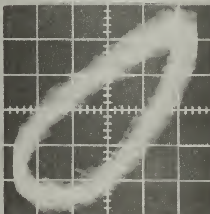
Fig. 17 Oscillograms of Phase Difference for freq. difference of 500 cycles
