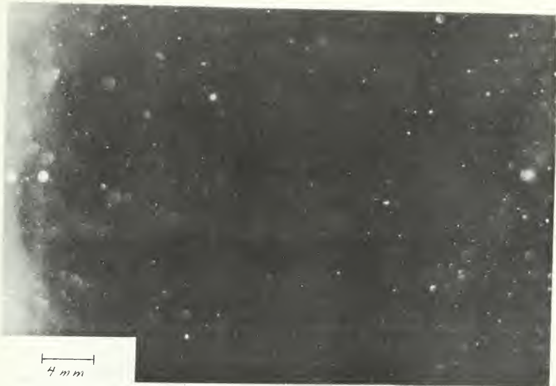
Figure IV-2(a). Photograph Showing the Effect of Scattering Caused by the Illumination of Bubbles Outside the Field of Focus.
