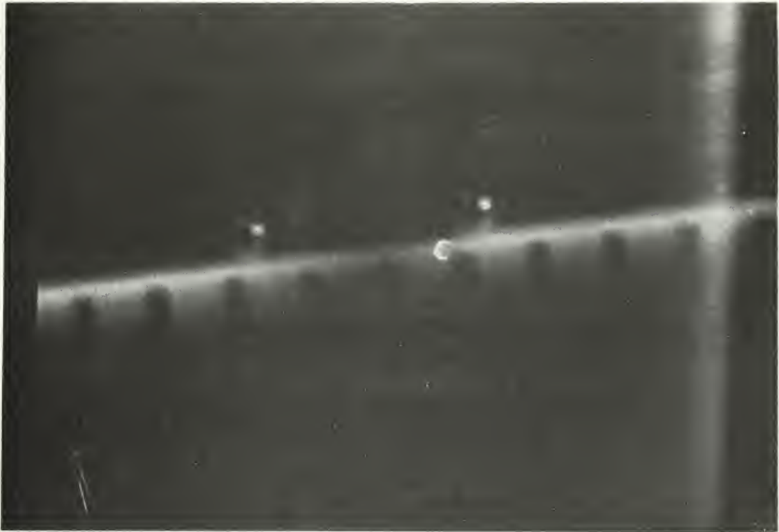
Figure IV-7. Photograph of Bubbles Suspended on the Edge of a Ruler. Markings are 1 mm Apart.
