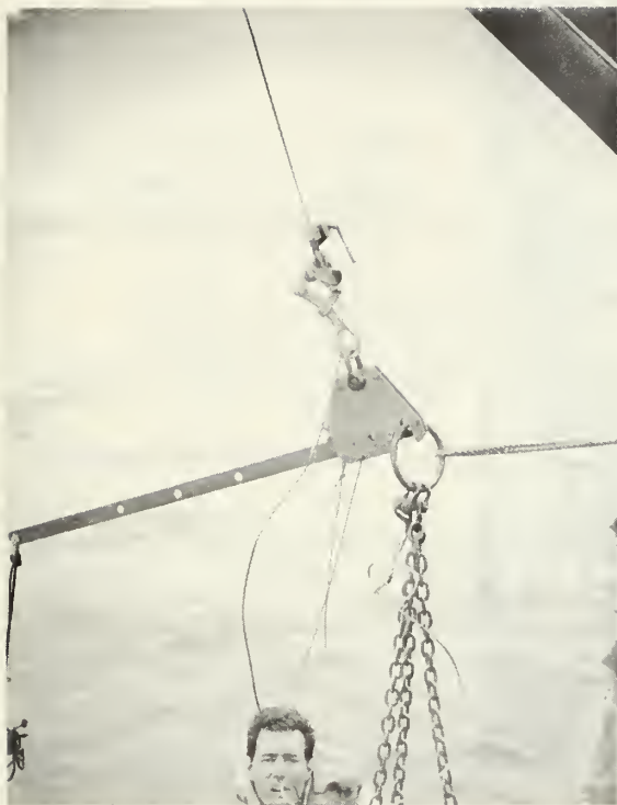
Figure 15. Release Mechanism In-Place on Wire Ready for Lowering
