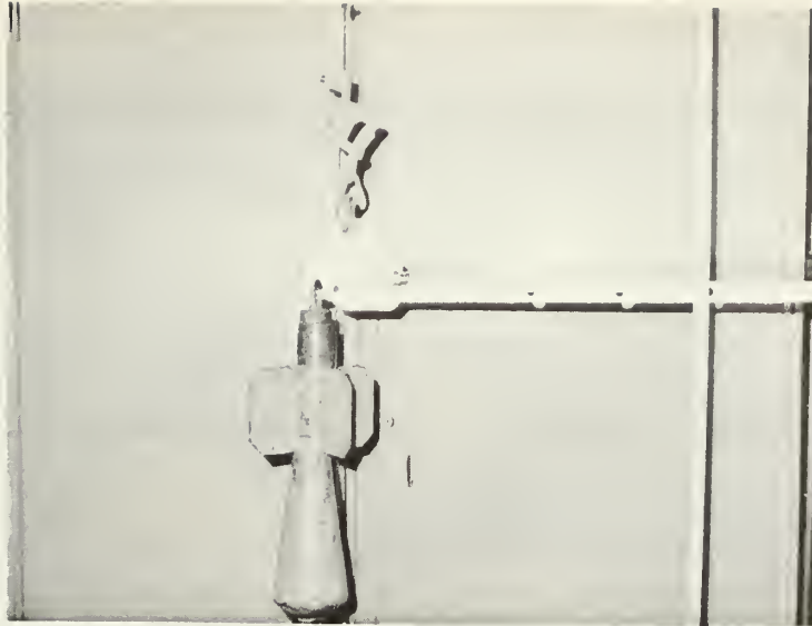
Figure 6. Release Mechanism and Drive Weight on Test Wire
