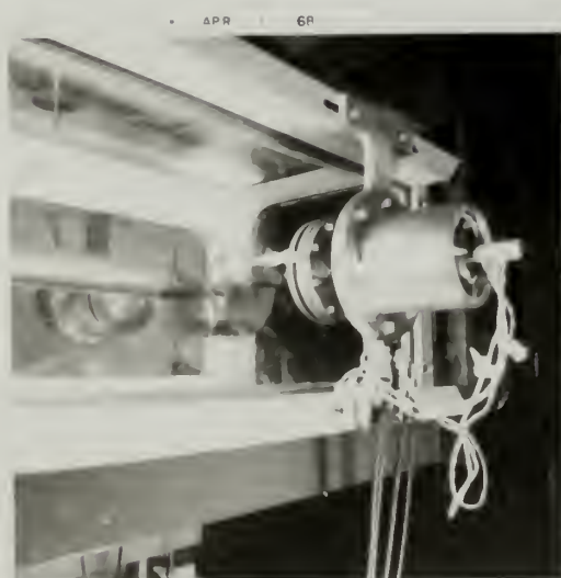
PROPELLER TUNNEL TEST SECTION WITH APPARATUS IN PLACE
