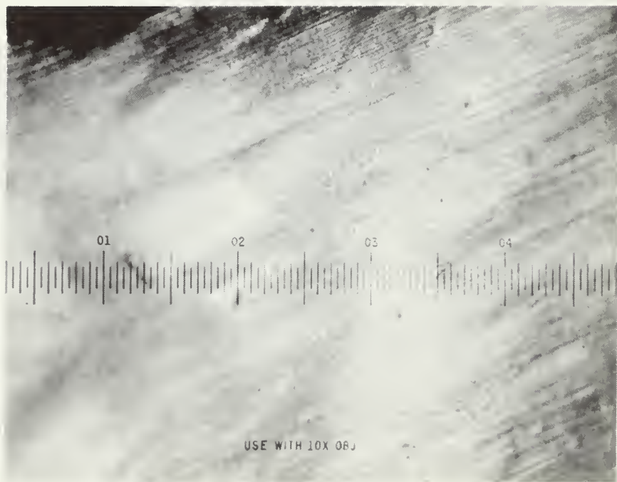
DEPOSITED PLASMA FROM .005 in. DIAMETER GOLD WIRE FIGURE 19
