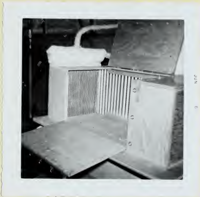
Figure A-7 View of Model Boiler With Doors Open
