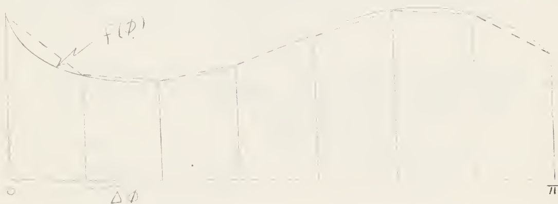
Trapezoidal Technique of Integrating Under a Curve by Summation
