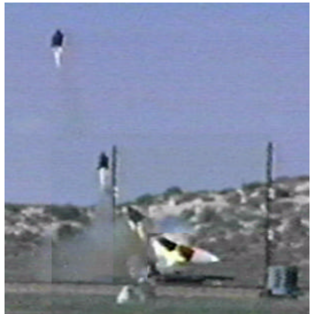
Figure 9.14 Multiple Exposure of Ejection Test from 60 deg Roll
