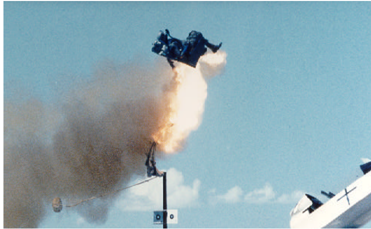
Figure 9.3 ACES II Ejection at 30 deg Pitch Angle
