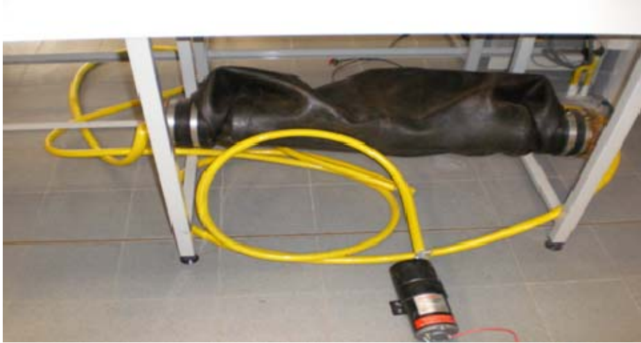
Figure 20. Expansion bladder for main ballast and associated tubing.
