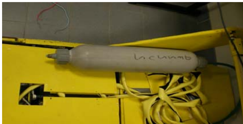
Figure 21. Compression bladder for main ballast.
