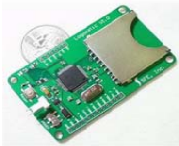
Figure 32. Universal Data Logger holding SD memory card. From (Sparkfun)
