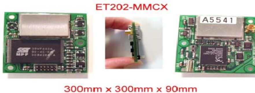
Figure 25. ET-202 GPS Receiver Engine Board. (from SparkFun)
