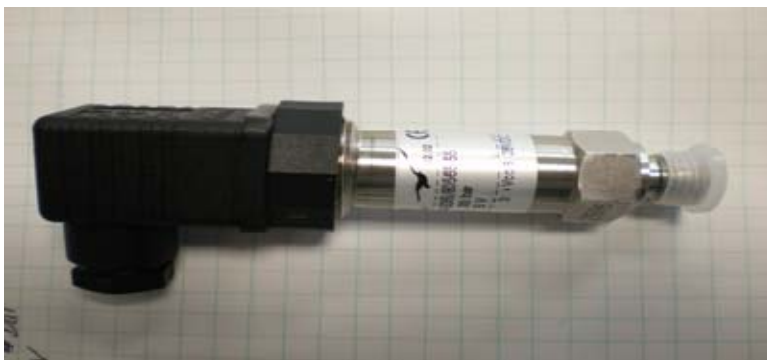
Figure 31. Keller-Druck Piezoresistive Depth Transmitter.
