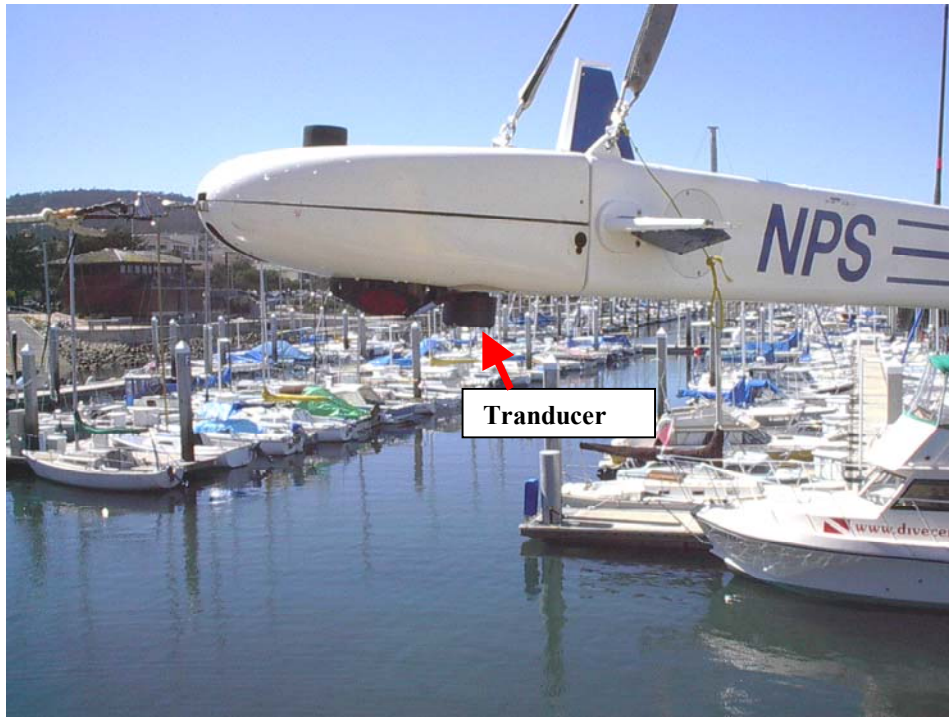
Figure 49. Benthos Modem Transducer Mounted on ARIES
