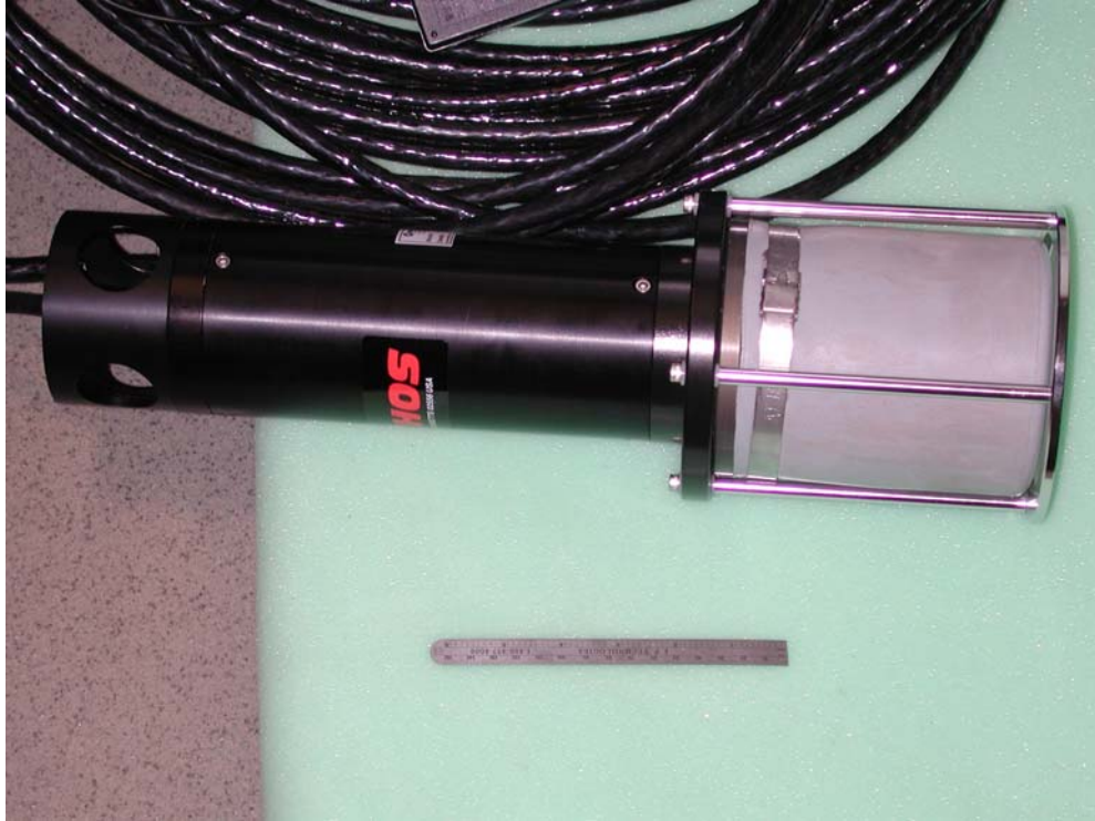
Figure 51. Benthos LF Transducer and 25 Meter Cable
