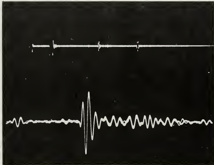
Figure 4.3 Reflected Pulse from Flat, Stirred Sand 1 cycle at 100kc. Normal Incidence
