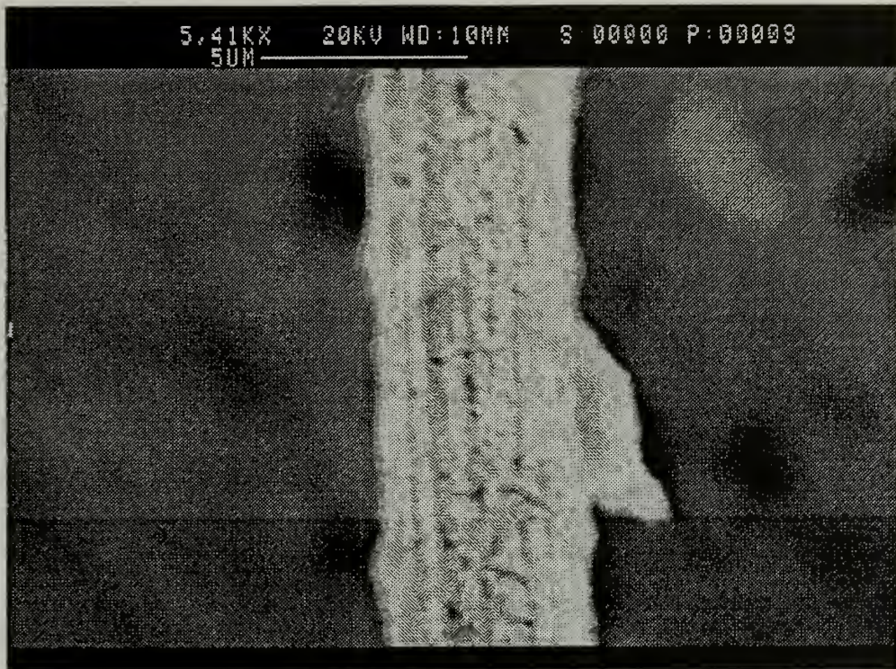
Figure 5-5: SEM image of striations and small bare patches (30 May 97).
