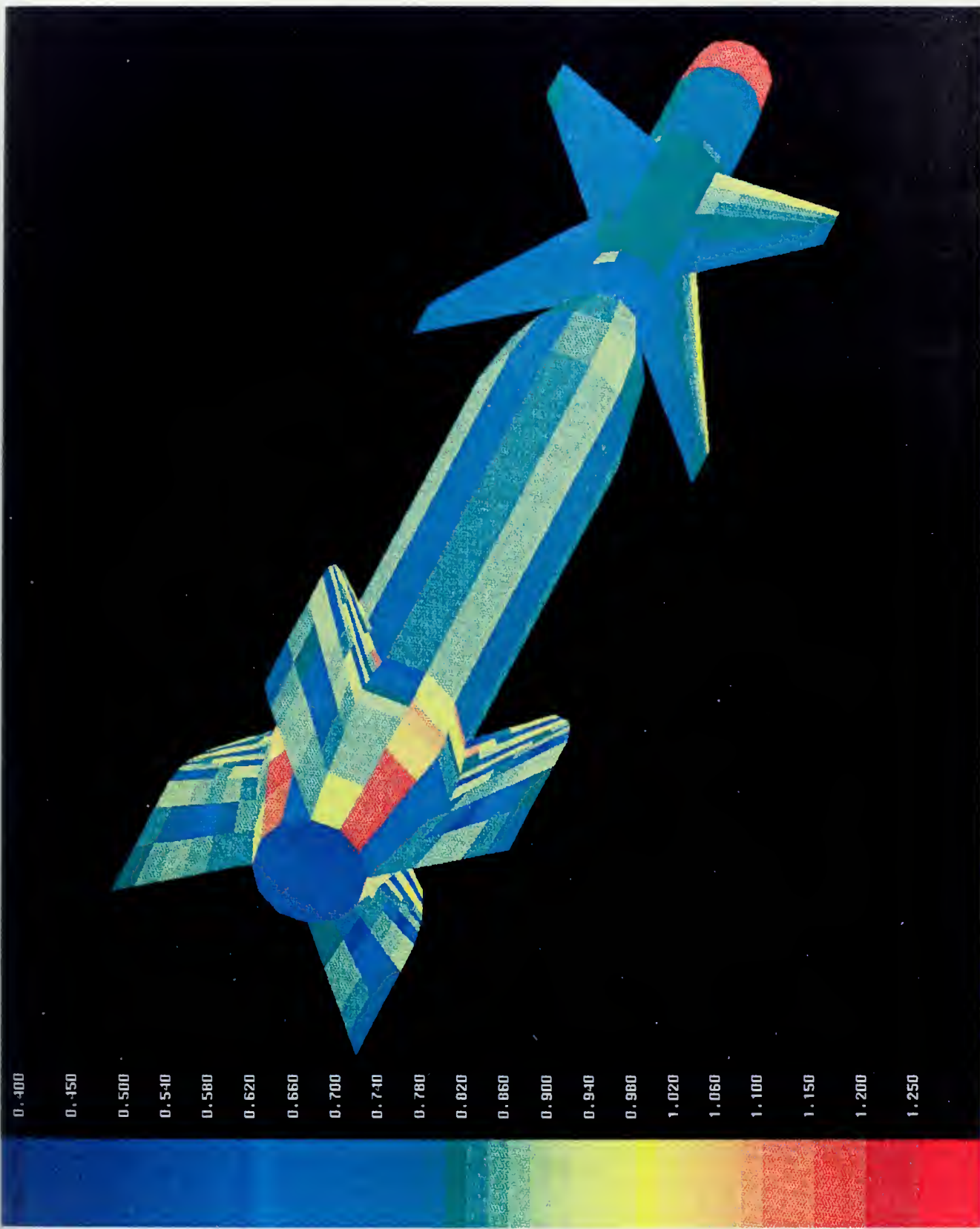
Figure 4.17 Mach Distribution over GBU-24 ( M_\infty=0.8 , \alpha=4^\circ )
