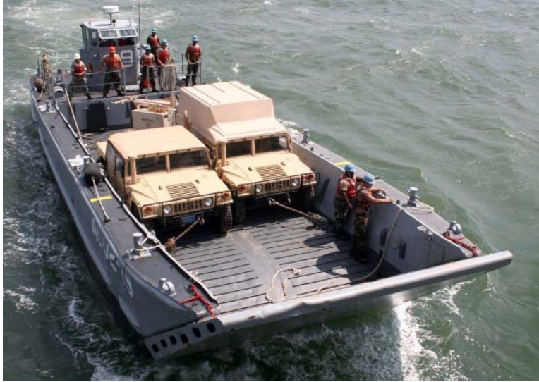
Figure 65. Landing Craft Mechanized (LCM-8) 279
