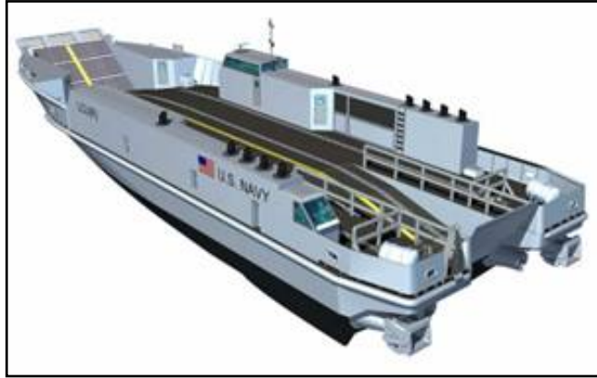
Figure 12-10: Landing Craft Utility, Replacement (LCU(R)). 273
