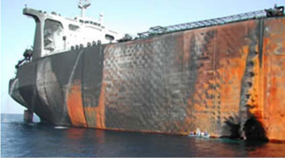
Figure 5. Damage to the French Tanker LIMBURG, October 2002
