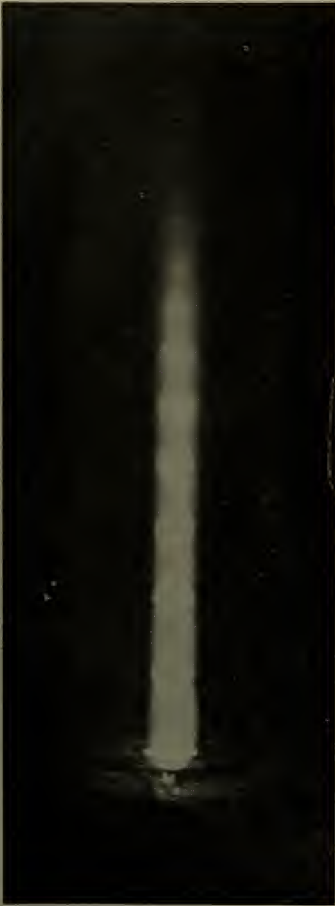
FIG. 10 HIGH-PRESSURE-SHOCK DIAMONDS IN HIGH-TEMPERATURE PRODUCTS OF COMBUSTION
