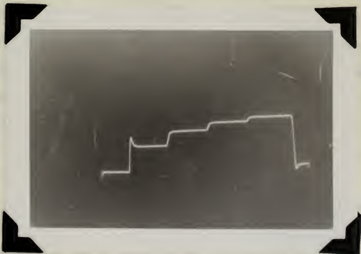
Figure II-8. "Staircase" Waveform at J12A. (Cathode Follower V8 removed to simulate all digit pulses present).
