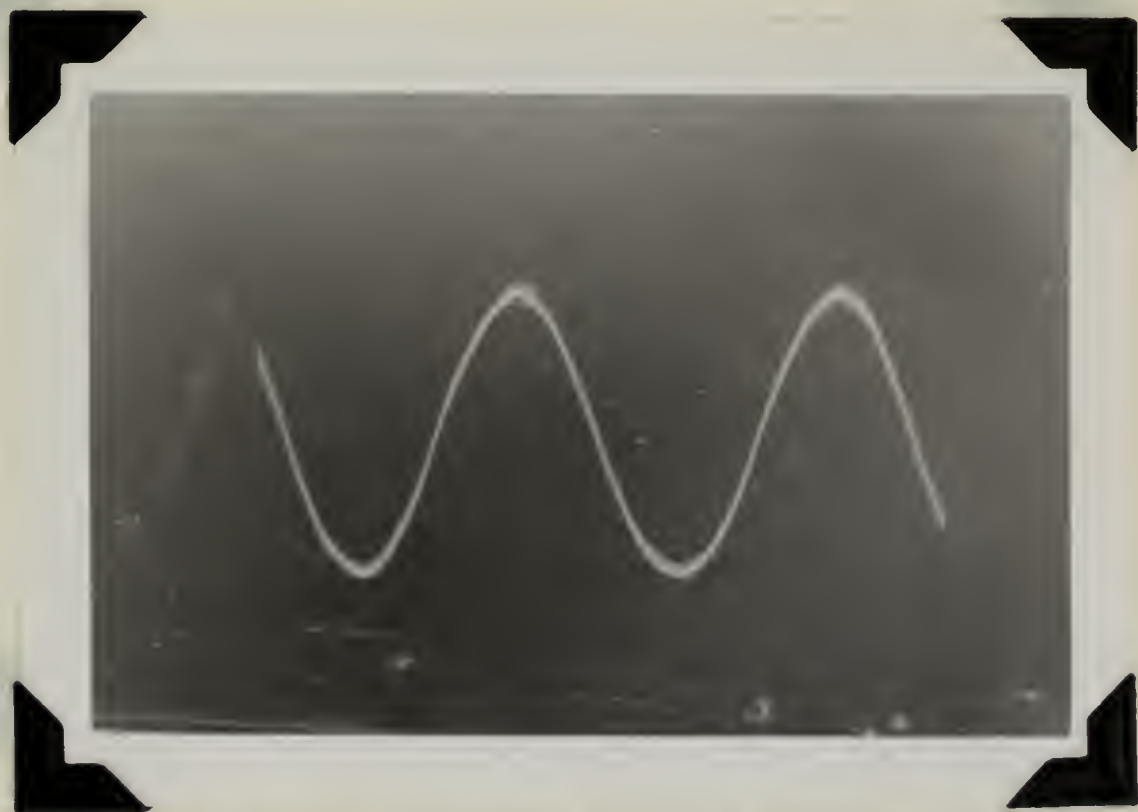
Figure II-14. 32-Level Decoder Output after Filtering. (200 c.p.s. sine wave input to coder).
