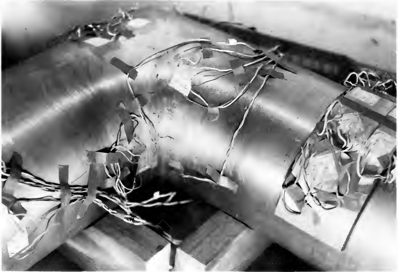
Fig. 4 Closeup view of second specimen showing rupture.
