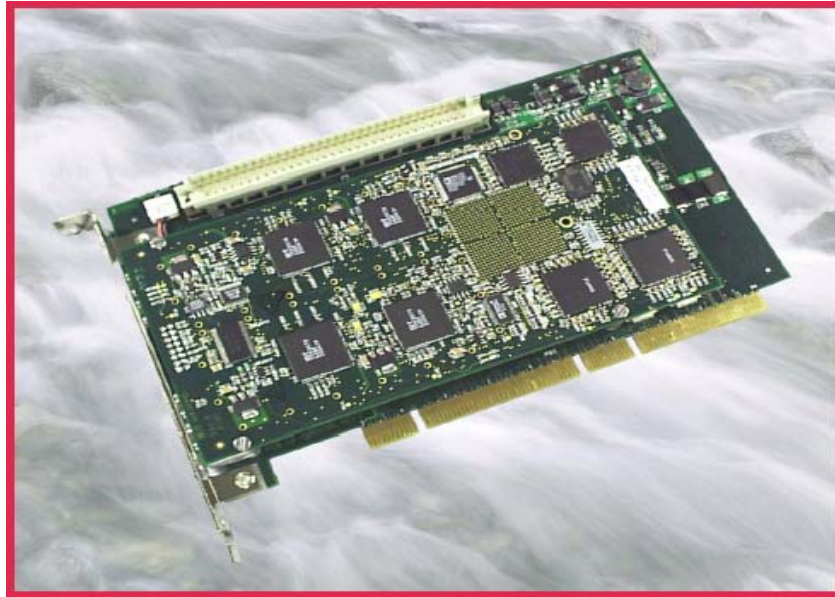
Figure 3-1. WaveRunner 253 PCI programmable SDR transceiver (From Ref. 7).
