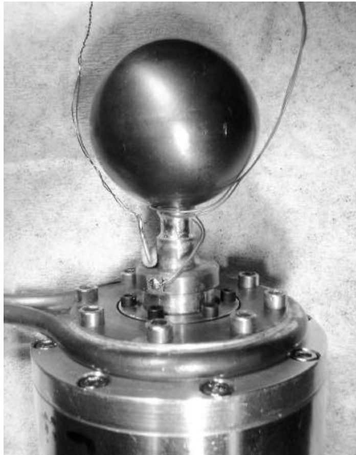
Figure 7.3. Location of the thermocouple on the cold heat exchanger with the leads at top-right, and the resistor on the cold heat exchanger with leads at top-left.
