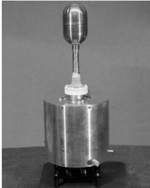
Figure 3.1. Brooks DemoTAR. The white is frost formed on the cold heat exchanger.
