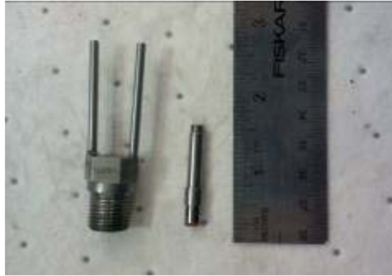
Figure 20. Kistler Pressure Sensor and Kistler Cooling Jacket (From [8])
