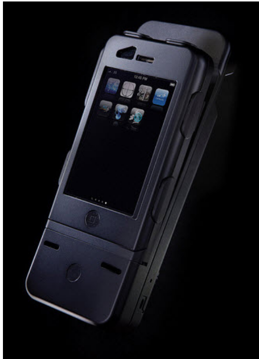
Figure 12. Handheld portion of the MONAX system with MONAX Lynx sleeve with COTS iPhone (From Lockheed Martin, 2010).
