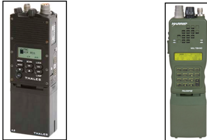
Figure 6. AN/PRC-148 V2(C) Multi-Band Inter/Intra Team Radio, (left) and AN/PRC-152 Multi-Band Multi-Mission Handheld Radios (right) (From Harris Corporation, 2011).
