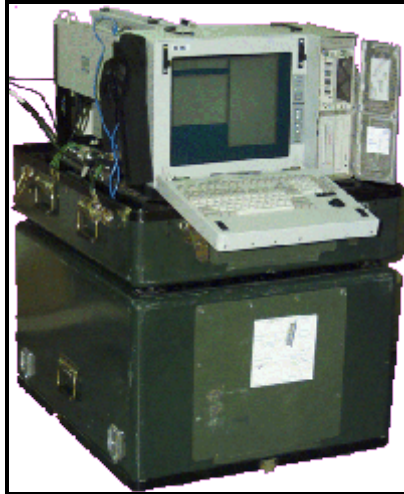
Figure 8. AN/GYK-47 (V) Advanced Field Artillery Tactical Data System (From PM FATDS, 2004).
