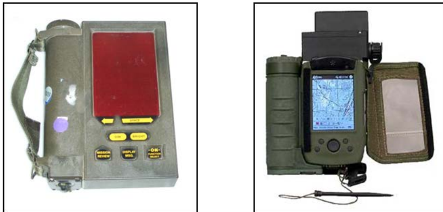
Figure 7. On the left the AN/PSC-2 Digital Communications Terminal (From Ebay, 2011) and on the right the AN/PSC-13 Dismounted-Data Automated Communications Terminal (From Scott, 2006).
