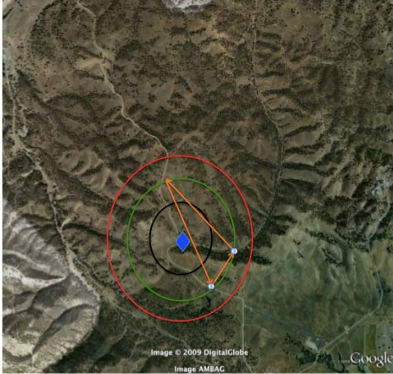
Figure 4: Varying radii flight paths for the UAV with predefined flight profile (orange) based on 750 m radius from the FOB
