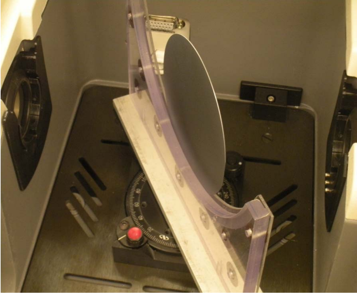
Figure 19. Experimental Setup for Measuring the Transmission of a Wafer
