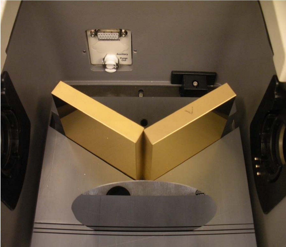
Figure 23. Experimental Setup for Measuring the Reflection of a Wafer
