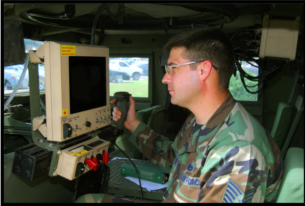
Figure 15 USAF airman demonstrating the CROWS weapon control station inside a HMMWV (From [20])
