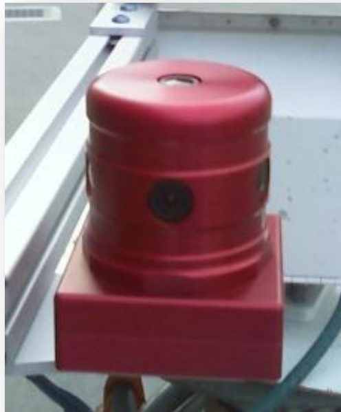
Figure 33 Ladybug® 2 spherical camera
