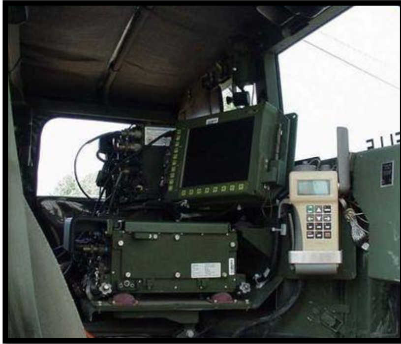
Figure 5 FBCB2 hardware mounted in a HMMWV (From [3])
