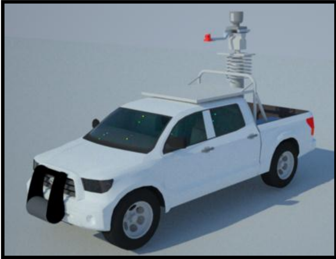
Figure 30 The PARPICE vehicle (rendered). Note the LiDAR and panoramic camera atop the telescoping mast.
