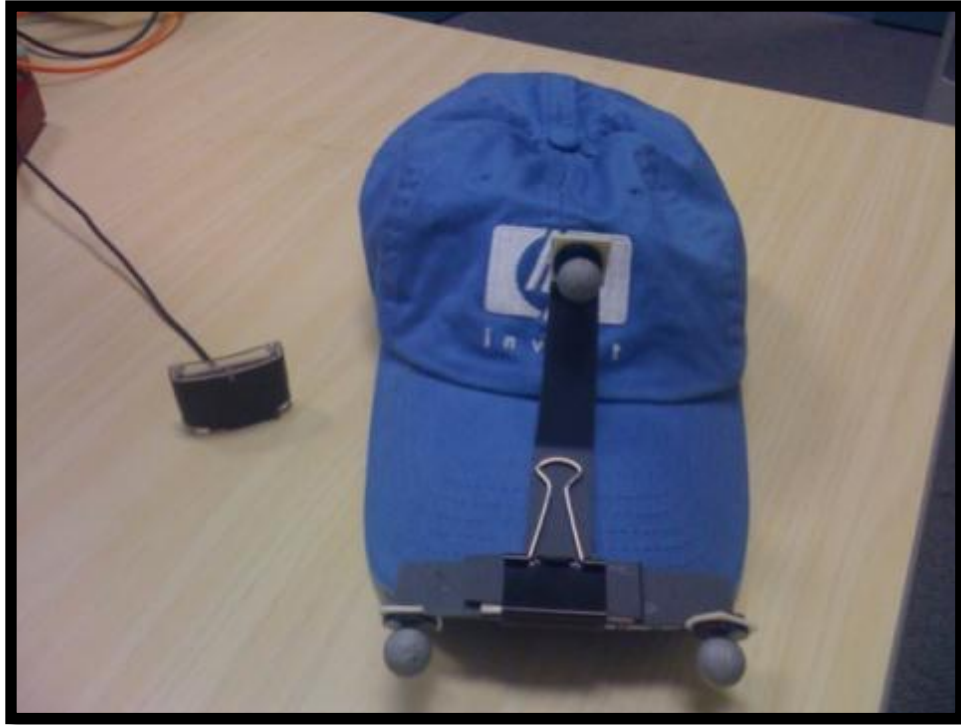
Figure 35 TrackIR™ camera and hat with reflective markers
