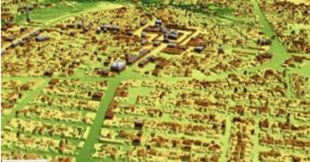
Figure 22 Model generated from LIDAR scan (from [34])
