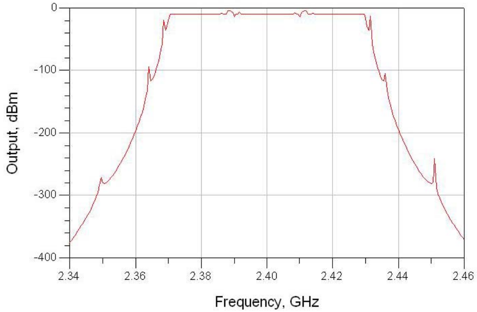
Figure 60. Output Amplitude Plot for the FDMC that uses Couplers and Butterworth Filters.
