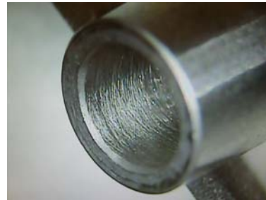
Figure 19.1 Test Specimen Samples Before Press-Fit
