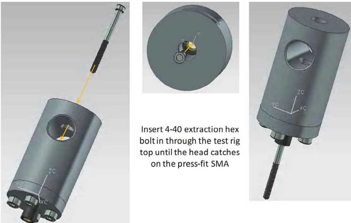
Figure 3.8 SMA 2 C Micro-Coupling Load Test Rig Upper Assembly with Extracting Hex Bolt Insertion
