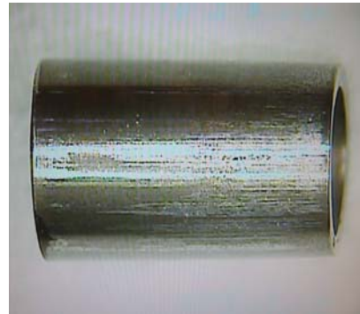
Figure 19.1 Test Specimen Samples Before Press-Fit
