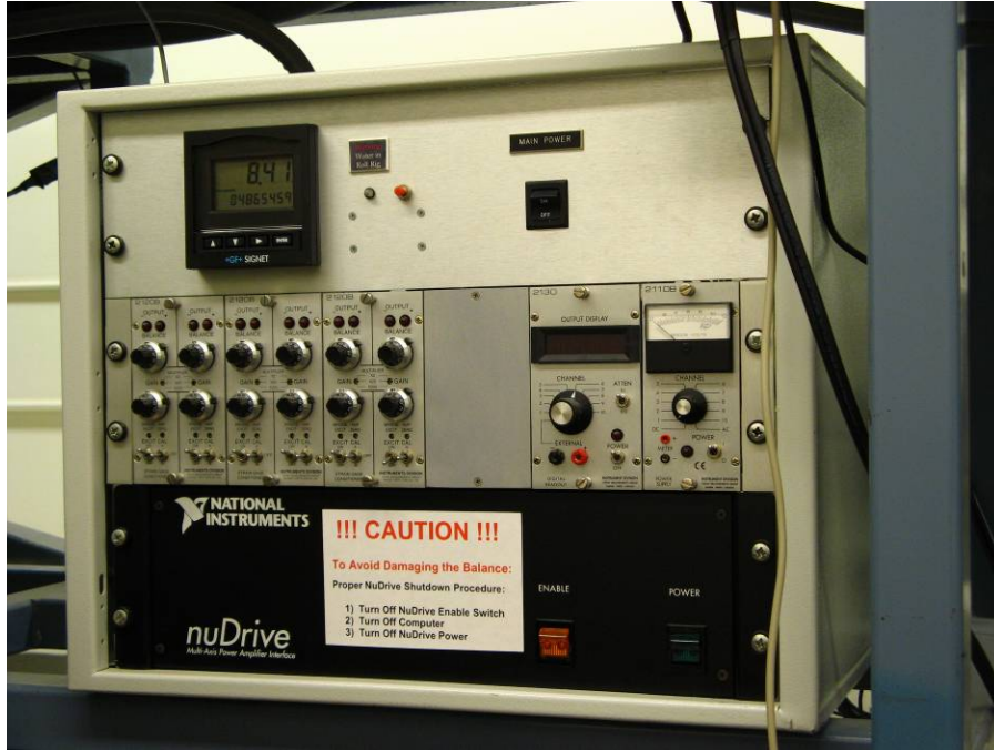
Figure 9. Control panel of NPS 15'' \times 20'' Flow Visualization Water Tunnel
