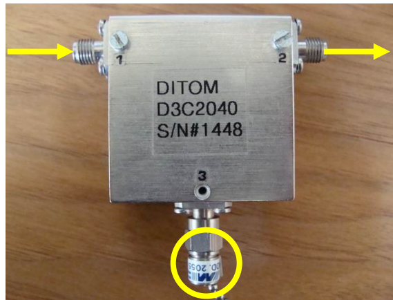
Figure 34. An isolator is inserted at the location of the LPA
