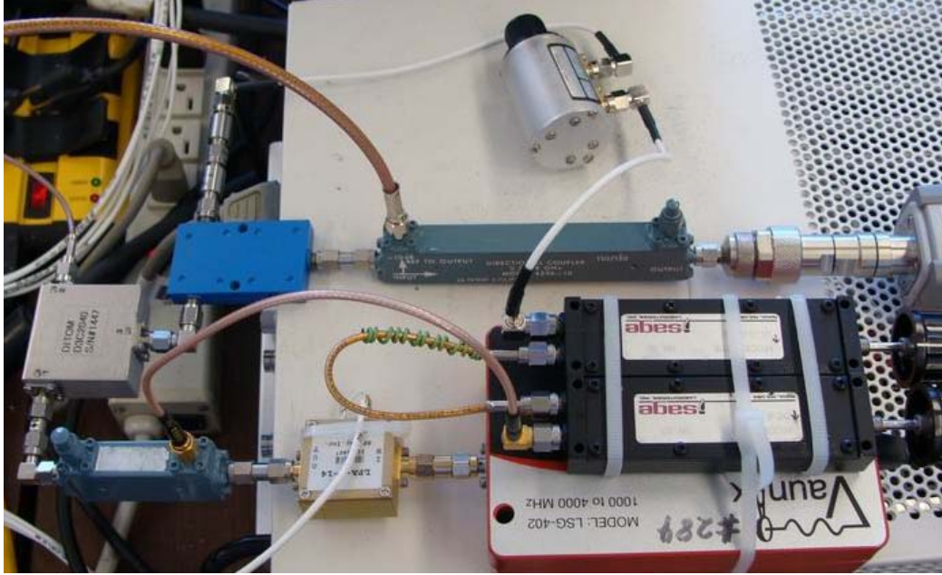
Figure 77. The appearance of the implemented leakage power cancellation circuit
