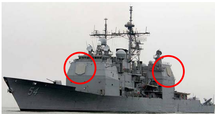
Figure 1. CG-54 with AN/SPY-1 radar highlighted (From [4])
