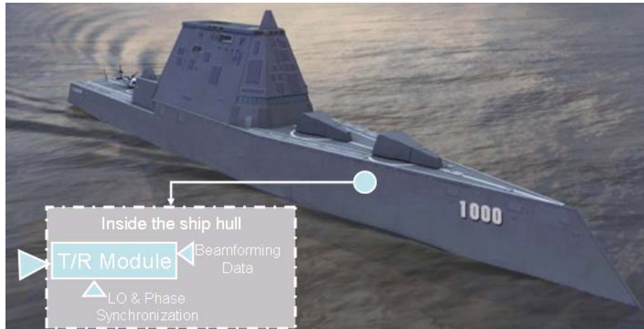
Figure 12. Configuration of WDDPA elements embedded in DDG–1000’s hull (After [29])
