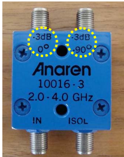
Figure 48. Anaren 3 dB quadrature coupler with the phase of the two ports highlighted
