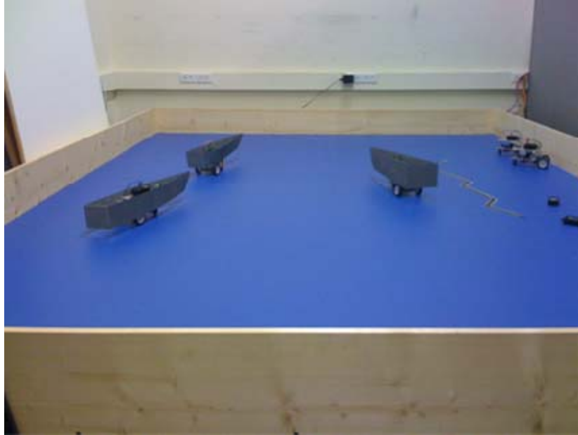
Figure 55. Maritime Training Table Prototype Created at NPS for EWD to Display SunSPOT-controlled Ship Models
