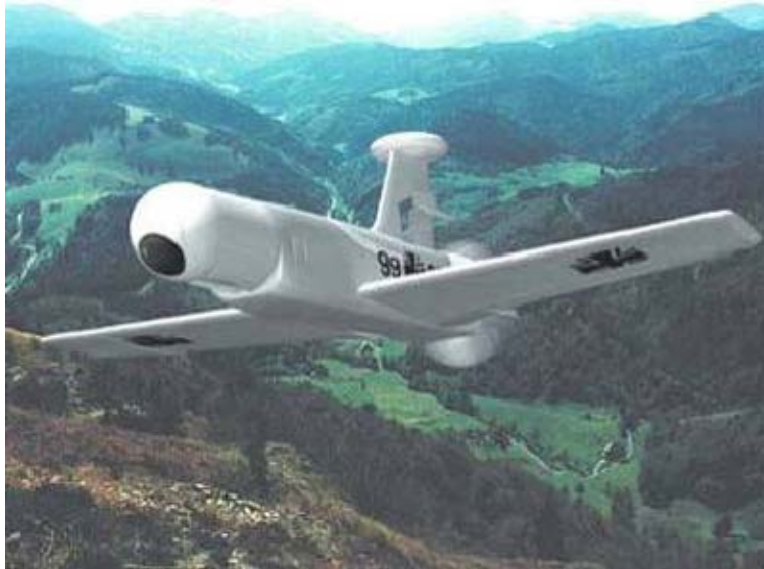
Figure 82. The Mücke electronic countermeasures (ECM) UAV (From [136])
