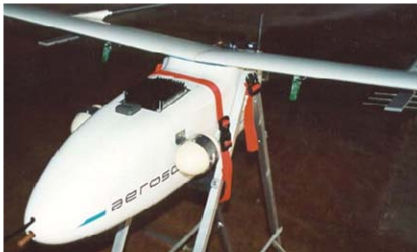
Figure 88. Aerosonde mini-UAV loaded with Antennas (From [144])
