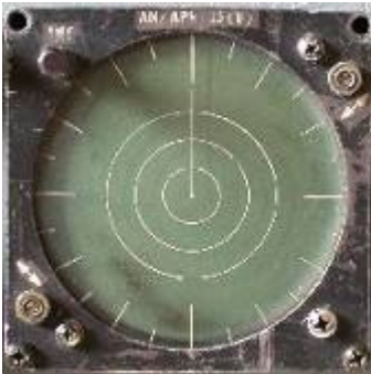
Figure 13. AN/APR-25(V) Strobe Display Scope (From[24])
