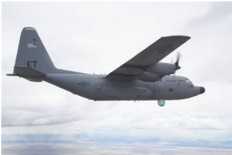
Figure 92. A C-130 Carrying An Advanced Tactical Laser (From [153])
