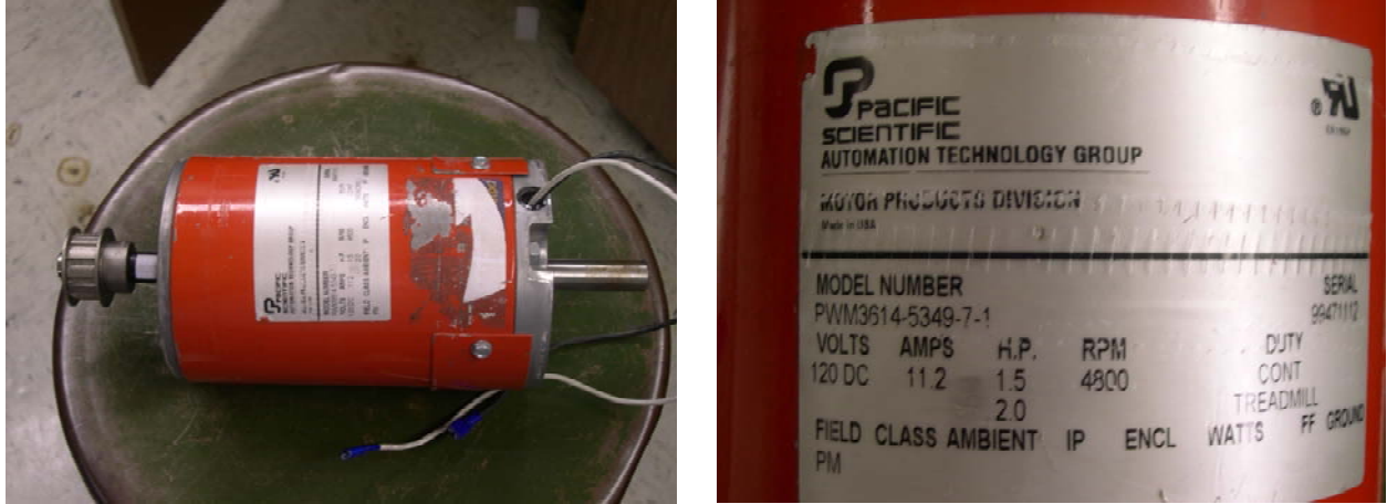
Figure 16: Bench Generator Prime Mover (1.5 HP)
