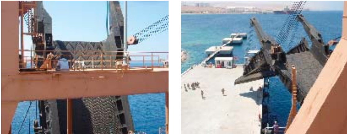
Figure 9. In both images, the RO/RO Ramp of the USNS Obregon attempts to descend upon the pier at Aqaba, Jordan.
