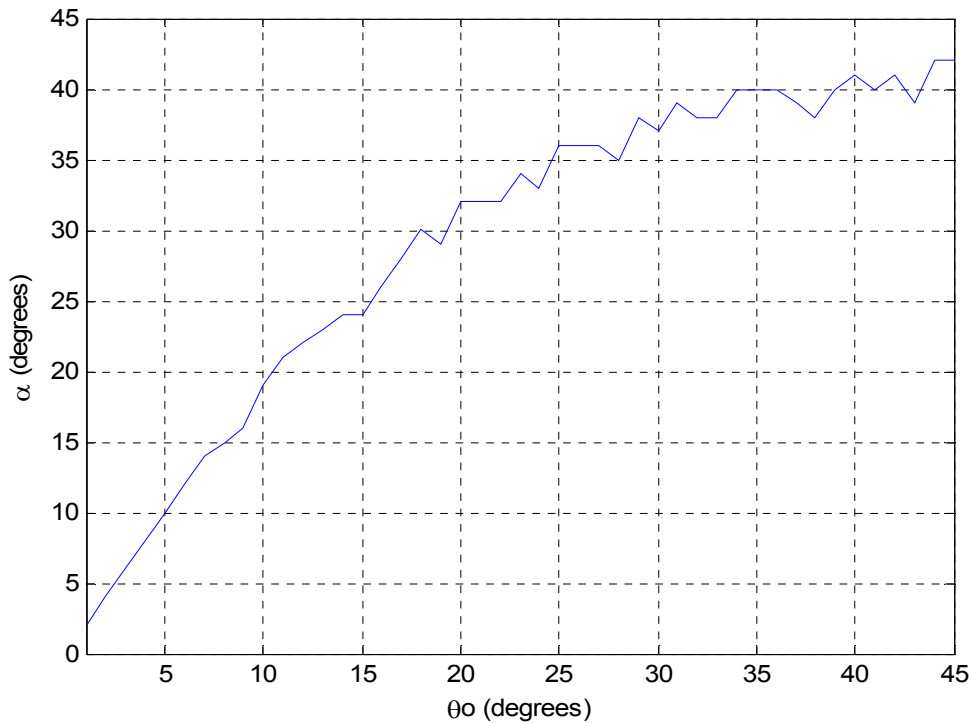
Figure 39. Characteristic angle producing the maximum tension for given \theta_0
