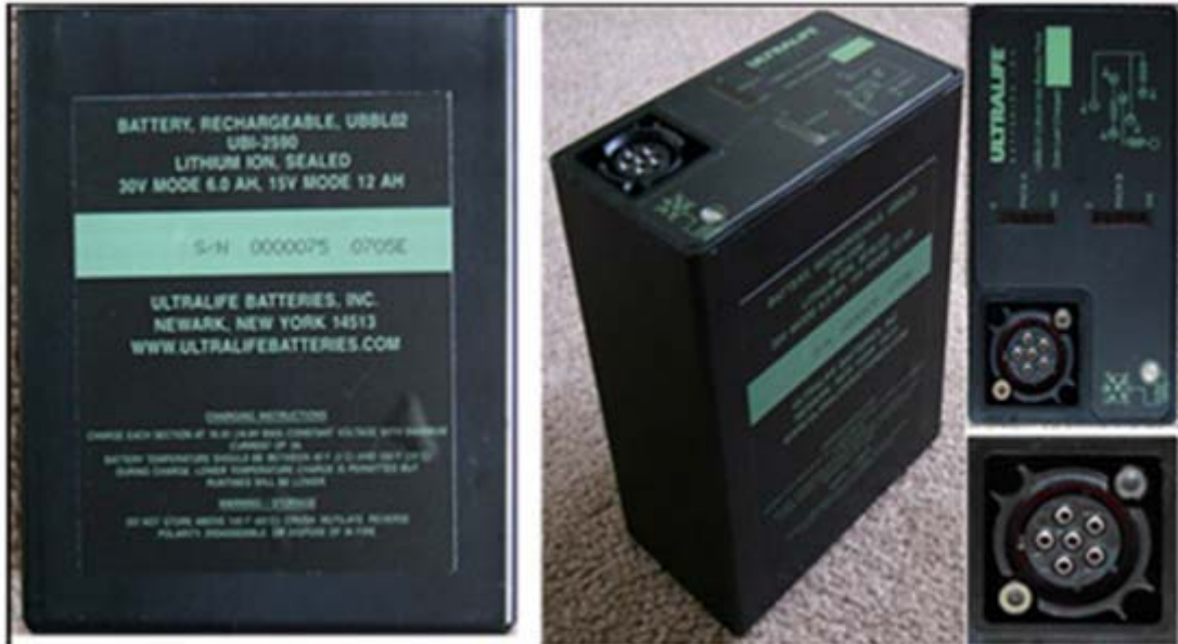
Figure 8. Ultralife UBI-2590 Battery
