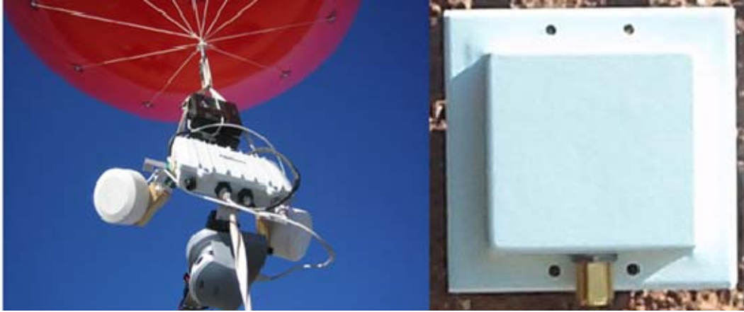
Figure 36. Aerial Payload and Antennas (Left Hyperlink Tech HG2408P 8dBi; Right SuperPass SPFPG9-V100 7dBi used on Balloon 1 in Figure 35 (From Superpass))
