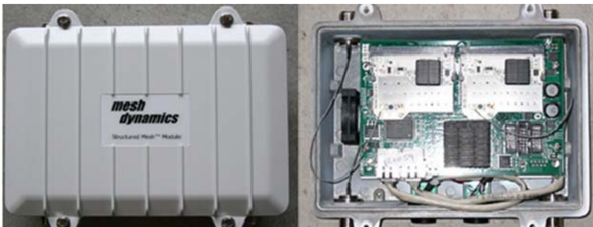
Figure 32. Mesh Dynamics Multi-radio Structured Mesh Network Access Point
