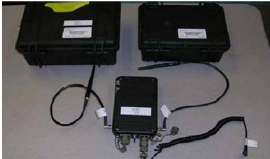
Figure 3. Rajant Technologies Breadcrumbs (XL, SL, ME) (From Lee 27)
