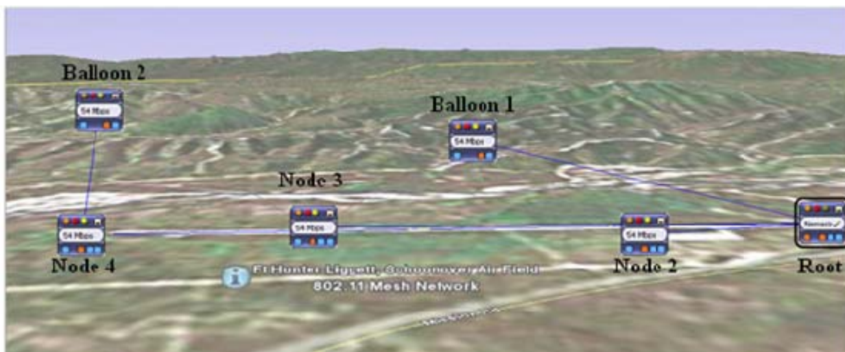
Figure 35. Topology at Ft Hunter Liggett (Test implementation of the proposed COASTS 2006 Thailand topology) (Background From Google Earth)
