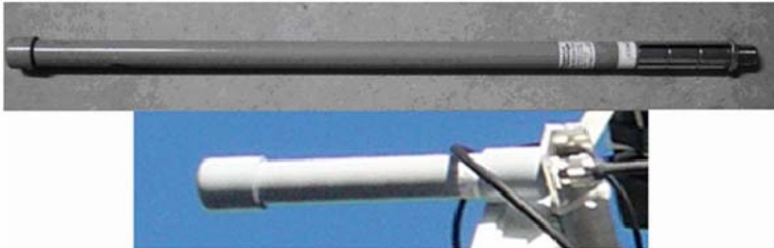
Figure 33. Backhaul Antennas Tested at Pt Sur (Top - Hyperlink 12dBi, Bottom - SuperPass 8dBi)
