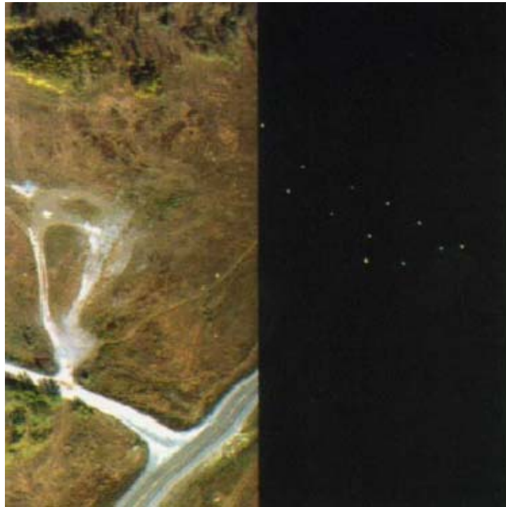
Figure 3. Surface-laid mine detections (From McFee and Ripley 1997).
