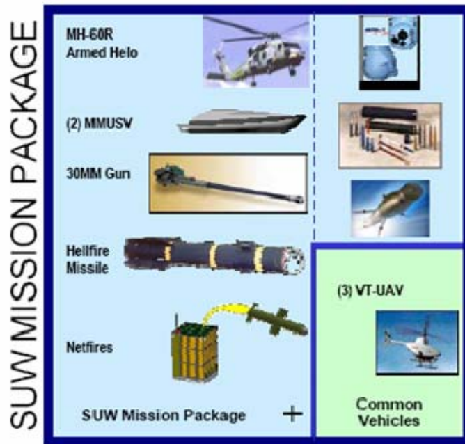
Figure 20. LCS SUW Mission Package Components [From Czapiewski] 68
