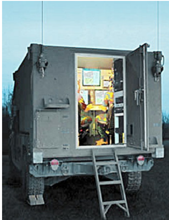
Figure 15. RQ-7 Shadow GCS Vehicle [From Jane's]
