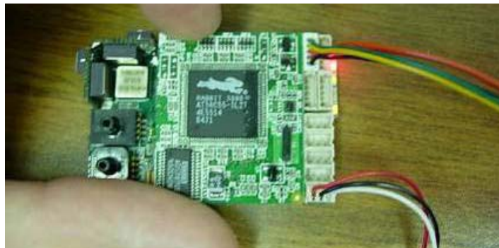
Figure 34. Connection for the programming and power cables on autopilot
