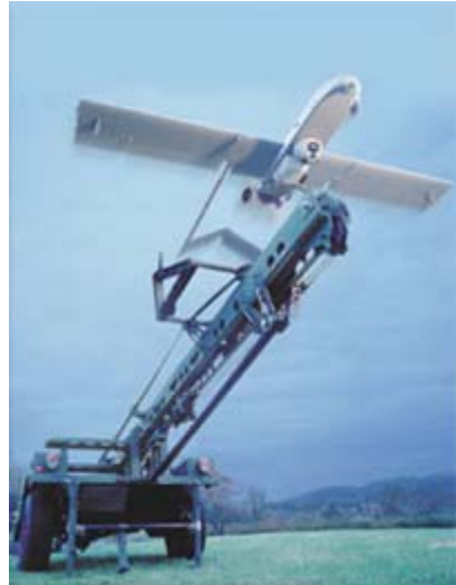
Figure 4. Shadow 200 being launched from a catapult
