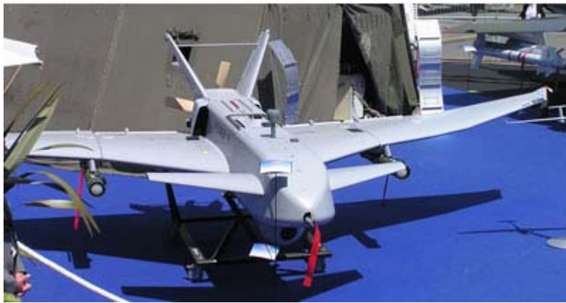
Figure 3. Sperwer B armed with Spike LR missiles
