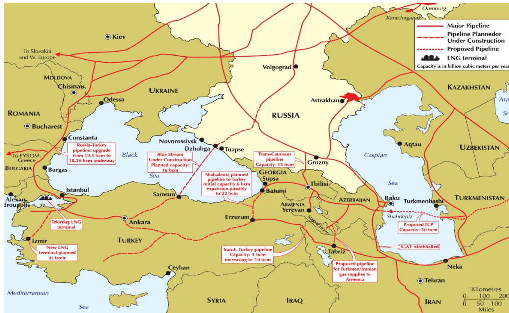
Figure 1. Existing and Projected Pipelines in the Transcaucasus (From: US Department of Energy, Energy Information Administration, Russia Energy Survey , 2002. Available from: http://eia.doe.gov/ (accessed 15 December 2005)
