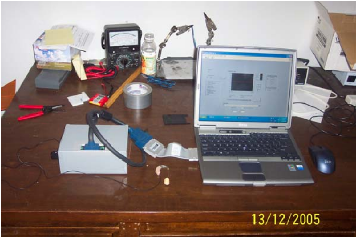
Figure 2.1. The complete set-up used for the recordings (ear microphone, A/D Converter, DAQ Card, and notebook with interface program).
