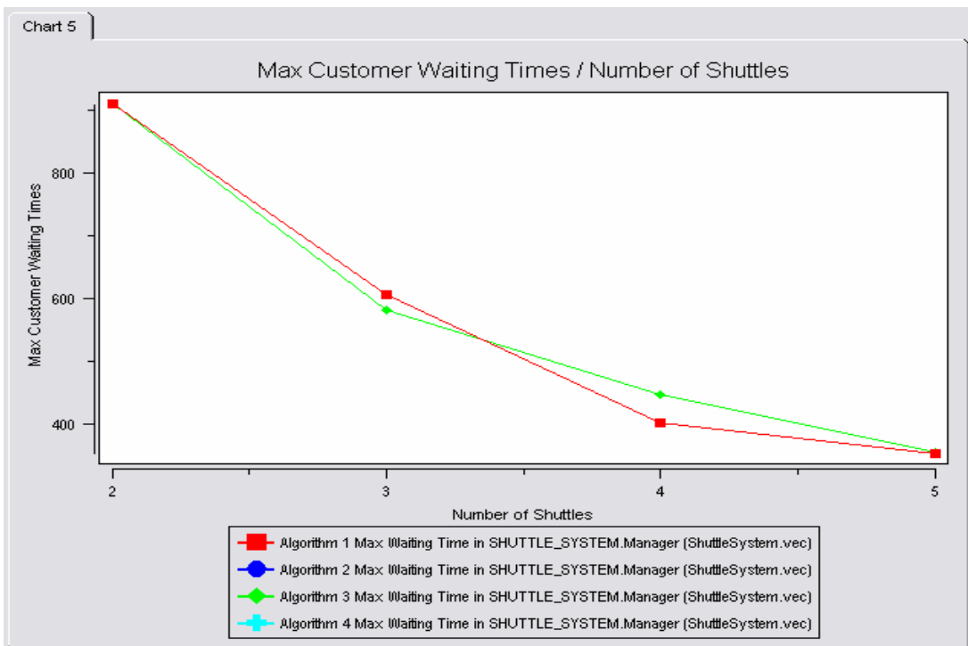
Figure 42. Visual Statistical Results of Experiment Six (Maximum Customer Waiting Times (seconds) / Number of Shuttles)
