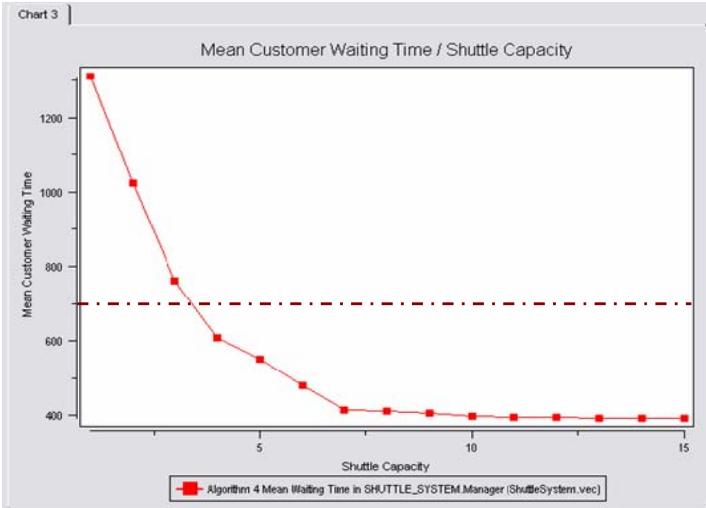
Figure 33. Visual Statistical Result of Experiment 5 (Average Customer Waiting Times (seconds) / Shuttle Capacity)
