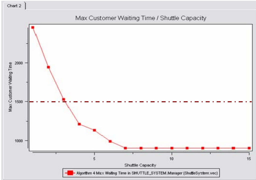
Figure 32. Visual Statistical Result of Experiment 5 (Maximum Customer Waiting Time (seconds) / Shuttle Capacity)
