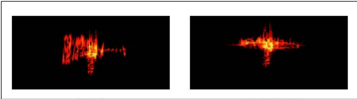
Figure 2 ISAR image improvement with motion compensation (From Ref. [11])
