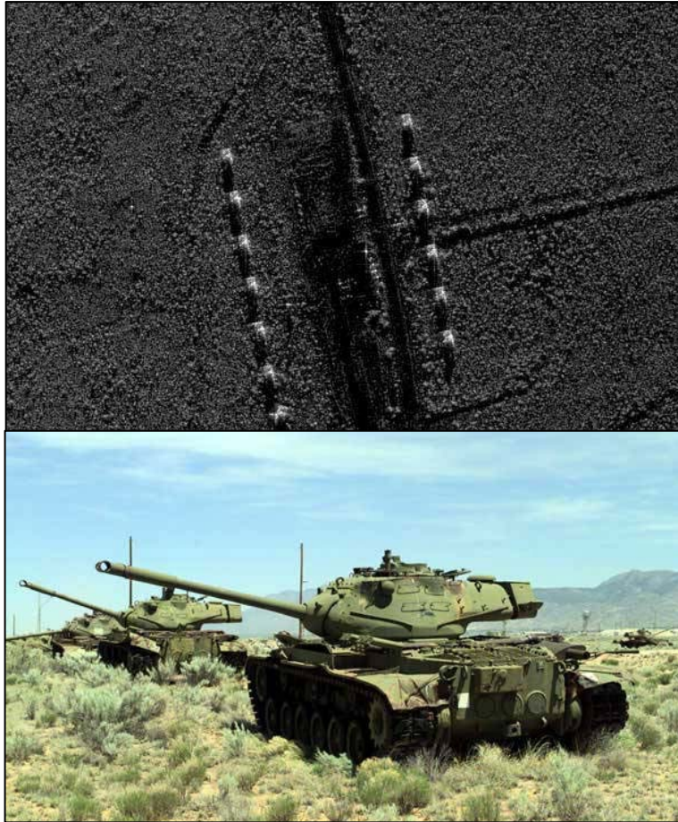
Figure 4 High Resolution SAR (above), compared to the optical image, to distinguish military targets (From Ref. [7])
