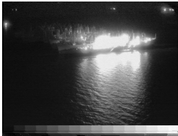
Figure 21. Flare Effect of Bright Lights on the Ships ( Photograph courtesy of Naval Research Laboratory)
