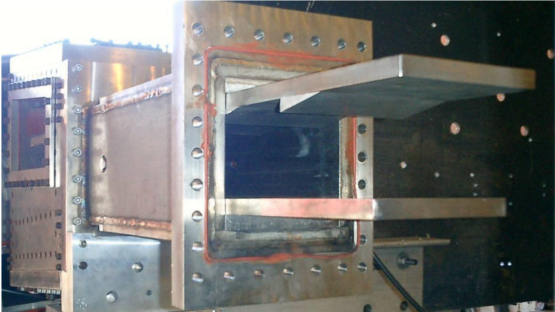
Figure 35. Transition Section Showing Removable Plates.
