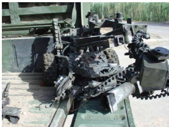
Figure 3. A robot destroyed by an IED in Iraq. (FY2005 JRP Master Plan)
