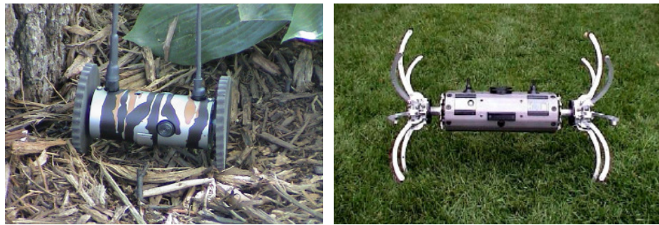
Figure 7. Left: A recent ThrowBot variant called the COTS-Scout. Right. A larger ThrowBot variant, the “MegaScout” with actuated-wheels (Kratochvil, 2003)
