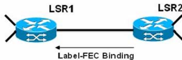
Figure 3. Downstream Unsolicited Label Distribution (From Ref. [9].)
