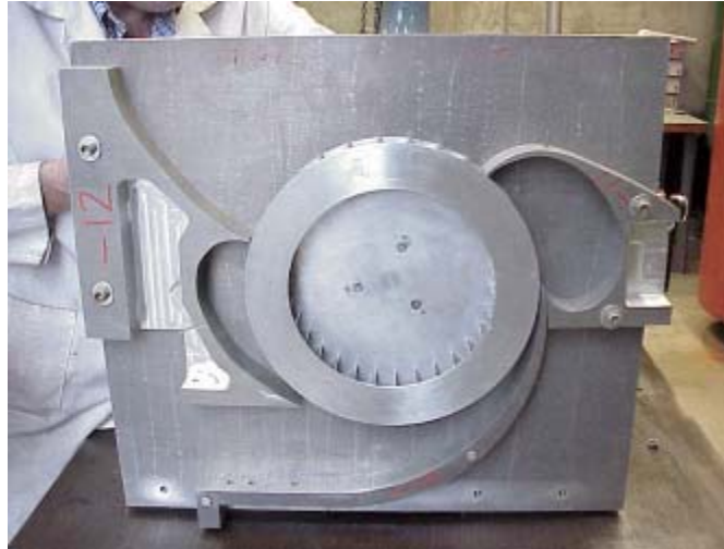
(c) Partially Assembled Figure 2. Cross-Flow Test Assembly (CFFTA, from Ref. 5)
